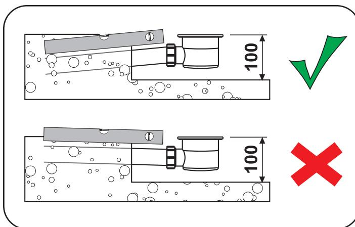
*In case that the manhole is larger than recommended, fill the manhole with 2K PU foam before installing the shower. PU foam after expansion must fulfill the manhole and be in contact with the bottom of the shower tray.*
